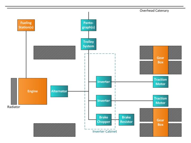
Off-board Trolley Assist adds additional parallel electric power source
