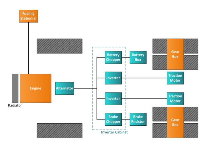
Unrestricted © Siemens Industry, Inc. 2017 Page 6 May 8, 2017 On-board Batteries provide additional parallel electric power source, energy storage
