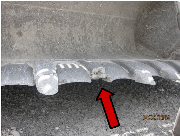
A tooth breaks off the loader.
