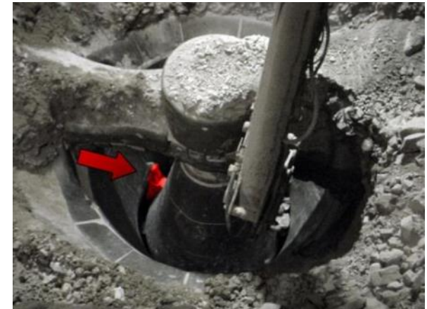
The tooth jams the crusher.
