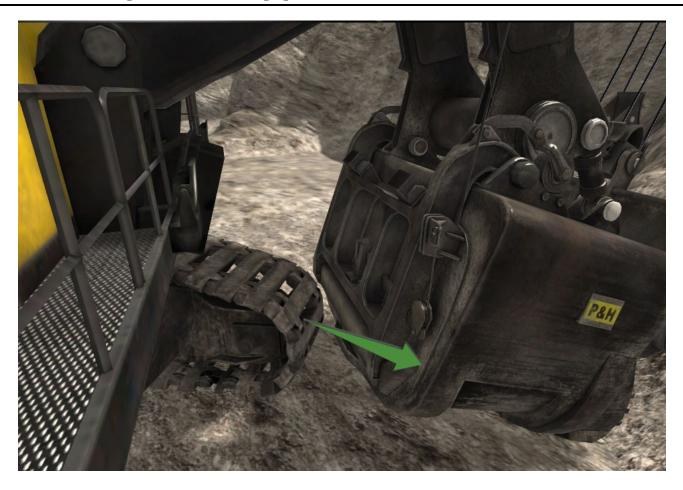
Current operation will not cause a collision between the dipper and the tracks so the Track Shield system no longer overrides the operator's hoist reference. With the autonomous assist active, the operator is able to move to the maximum "limit" and gets used to the muscle and visual memory.
