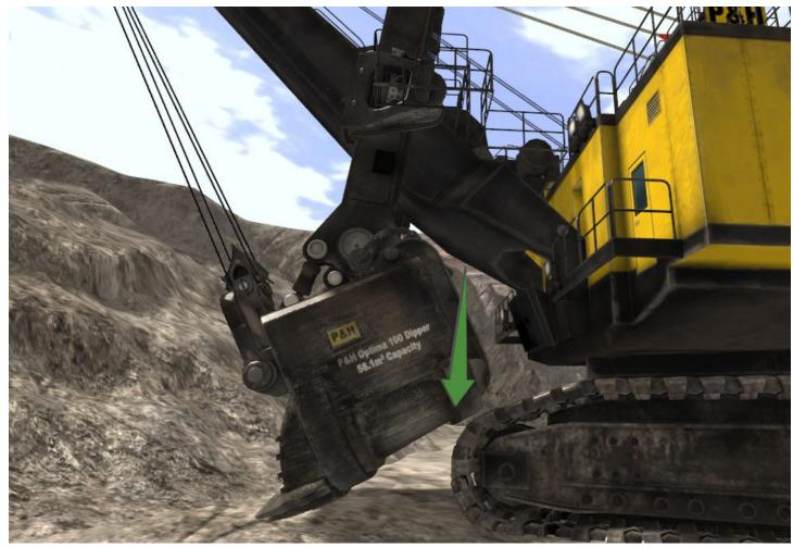
The Track Shield system identifies that the current operator commands may cause a collision between the dipper and the tracks but still does not attempt to override the operator's commands because of the slow speed being applied.
