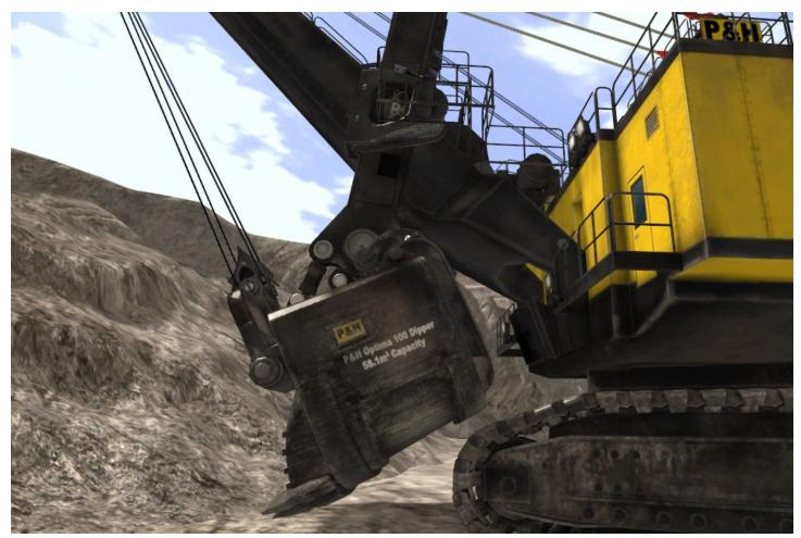
The Track Shield system does not detect any pending collision because the operator is not commanding any hoist, crowd or swing reference that may cause a collision. Therefore the Track Shield system does not override the operator's commands.
