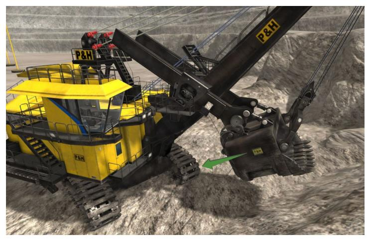
The Track Shield system identifies that the current operator commands may cause a collision between the dipper and the tracks but still does not attempt to override the operator's commands because of the large distance between the dipper and tracks.
