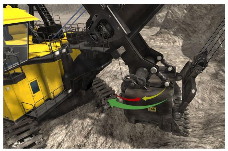
The Track Shield system identifies that the current operator commands may cause a collision between the dipper and tracks given the short distance between the dipper and tracks. The Track Shield system applies an overriding command that begins to reduce the hoist reference.
