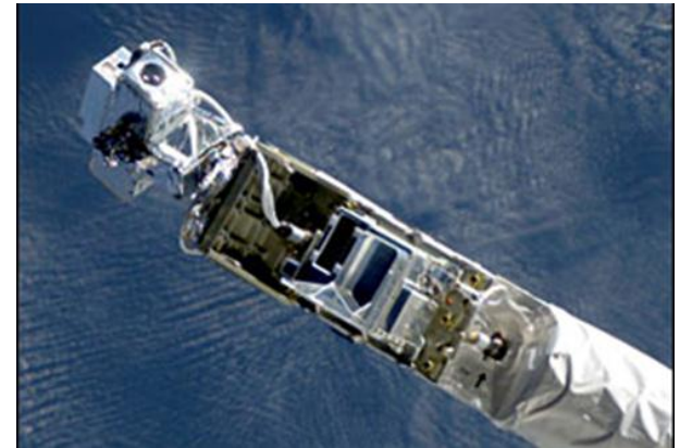
3D laser sensor to inspect the heat shield on the Space Shuttle
