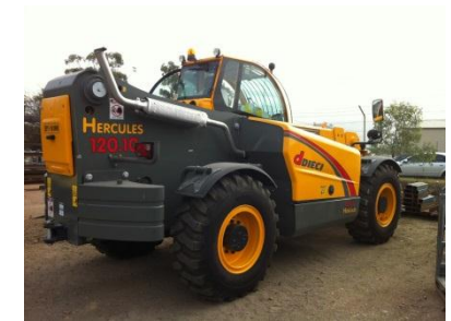
Dieci Hercules 120.10 mobile crane and forklift
